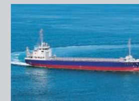
Hybrid Cargo Ship "Utashima" equipped with lithium-ion batteries
